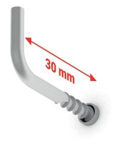
**8.** Then screw "L-hooks" in the wall plugs. However, make sure that hooks are not tightened too much. Their role is to ensure an equal position of the mirror which should be situated about 30 mm from the wall.
