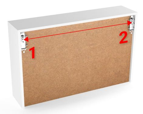
**2.** Using the measurements, mark two points on the wall with the centers of the hangers. Then put the mounting plates in the designated places and mark four points that will serve you to drill the holes.
