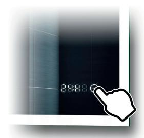
**4.** Then hold the switch for three seconds to activate the time setting mode. Select the right time by short pressing. In order to set minutes, hold the switch down again for three seconds. Use short press in order to set minutes.
